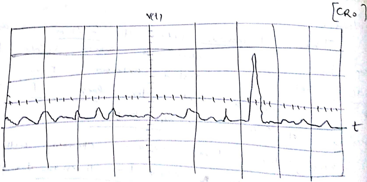
fig 2:- A spike superimposed on a background of smooth (thermal) noise
