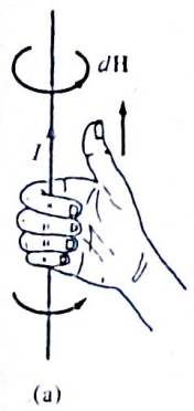
Figure 4.2 Determining the direction of dH using (a) the right-hand rule or (b) the right-handed-screw rule.
